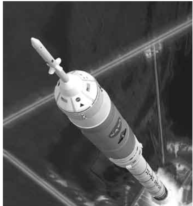
An artist concept of an Ares launch with the Orion crew capsule and the abort system in the tower on top.
