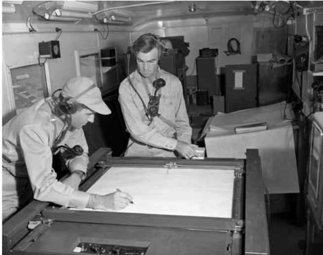
*A plotting board used to track the location of a missile in real time - inside a van or trailer.*
