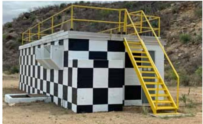
*The 100K blockhouse as seen today after WSMR's Cultural Resource Management Program recently refurbished the structure. This part of the building faced the test stand and it is 18 inches of reinforced concrete while the backside walls are cinder block construction. Photo courtesy Bill Godby.*
