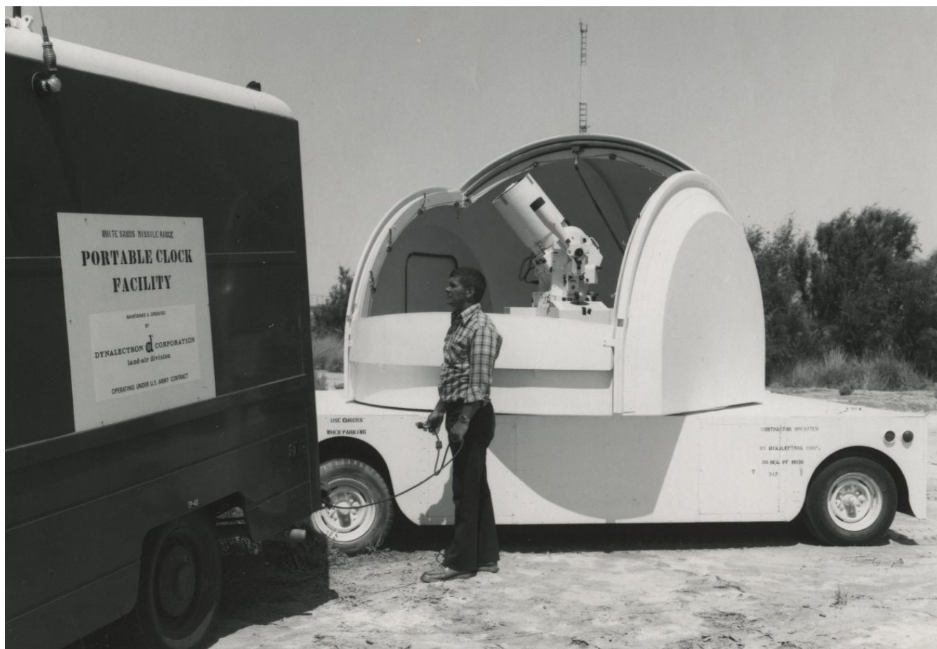
Figure 36. Portable clock van for mobile cinetheodolite, circa 1965 ( Jim Andress Collection, WSMR Museum Archives ).
