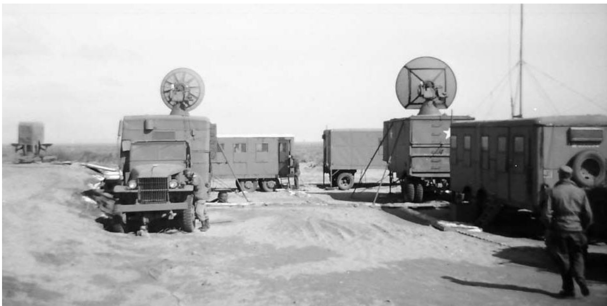
Figure 10. SCEL-modified SCR-584 radar units at C-Station in 1947 ( image courtesy David K. Barton ).
