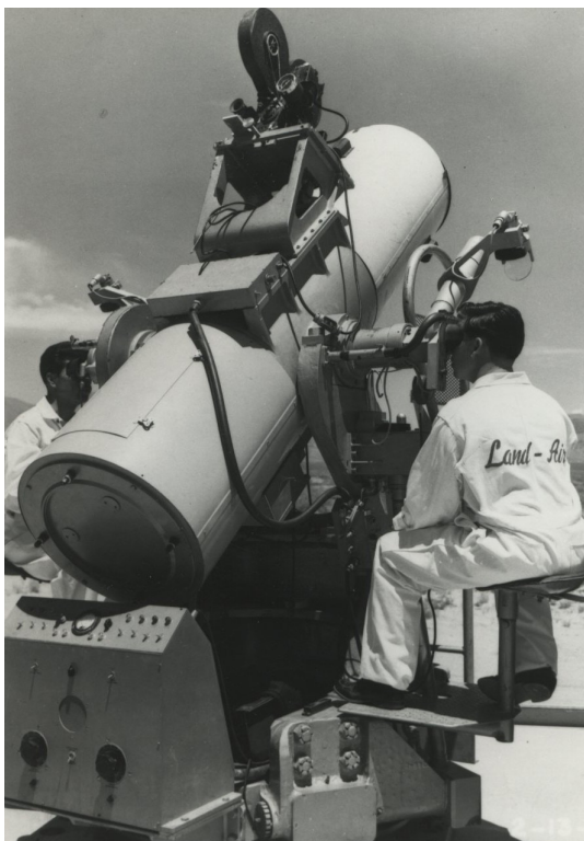
Figure 8. Land-Air staff manning a Modified Intercept Ground Optical Recorder (MIGOR) circa 1960 (courtesy WSMR Museum Archives).
