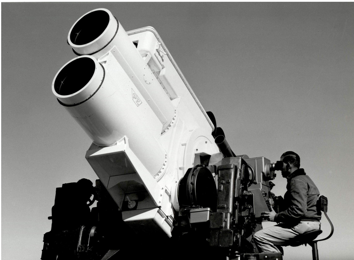
Figure 32. The ROTI Mk I optical instrument, circa 1959 ( courtesy WSMR Museum Archives ).
