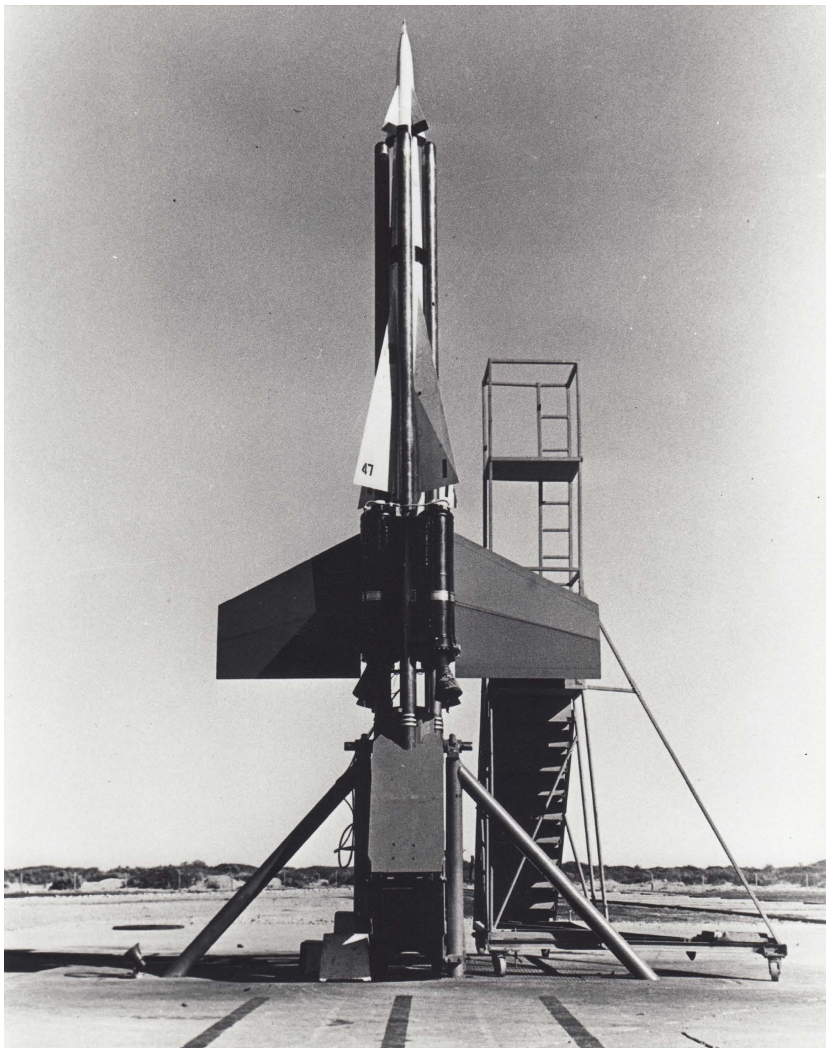
Figure 28. A Nike 47 missile installed on the quad rail launcher, circa 1947 (photo courtesy WSMR Museum Archives).
