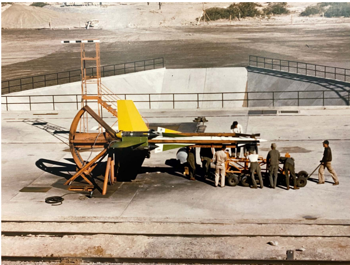
Figure 24. A Nike 46 missile installed on the original Nike rail launcher at LC-33, circa 1946 ( photo courtesy WSMR Museum Archives ).
