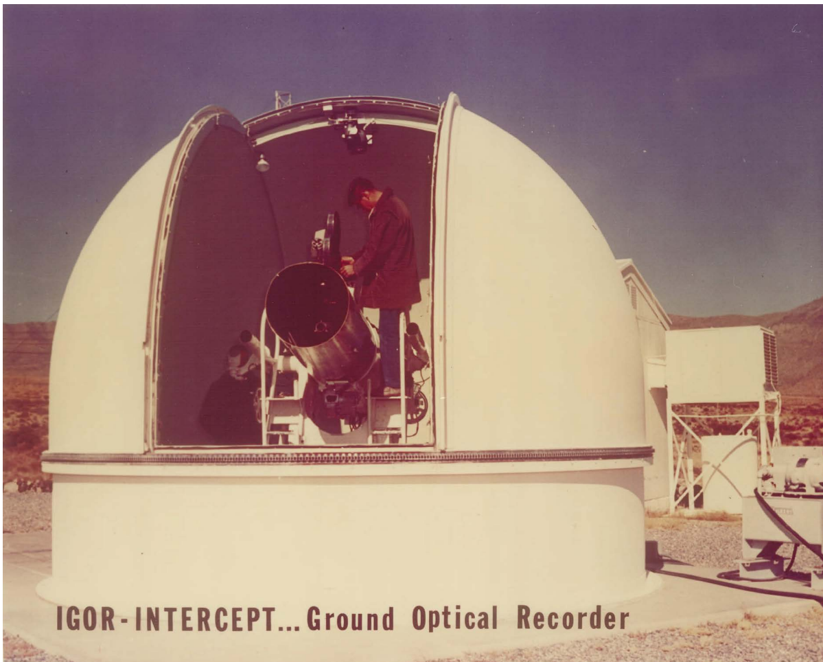
Figure 8. The IGOR tracking telescope housed in an astrodome, one of the new generation of specialized tracking instruments developed during the 1950s ( courtesy WSMR Museum Archives ).
