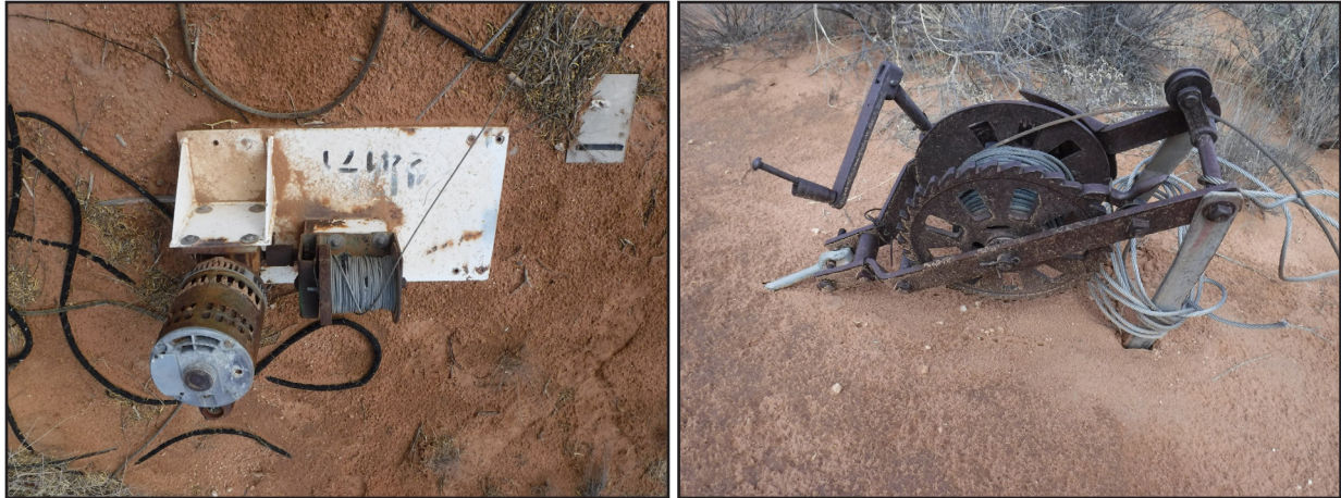
Figure 329. Property 24171, electric winch assembly with stenciled property number ( left ); manual winch attached to guy line anchor ( right ).
