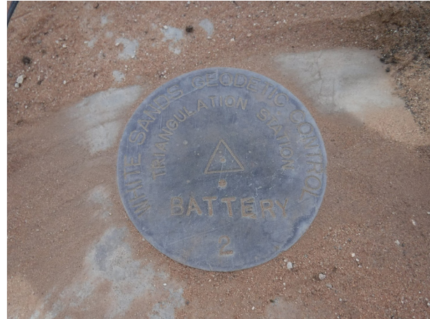
Figure 313. Property 23698, brass survey datum marked "BATTERY 2," plan view.
